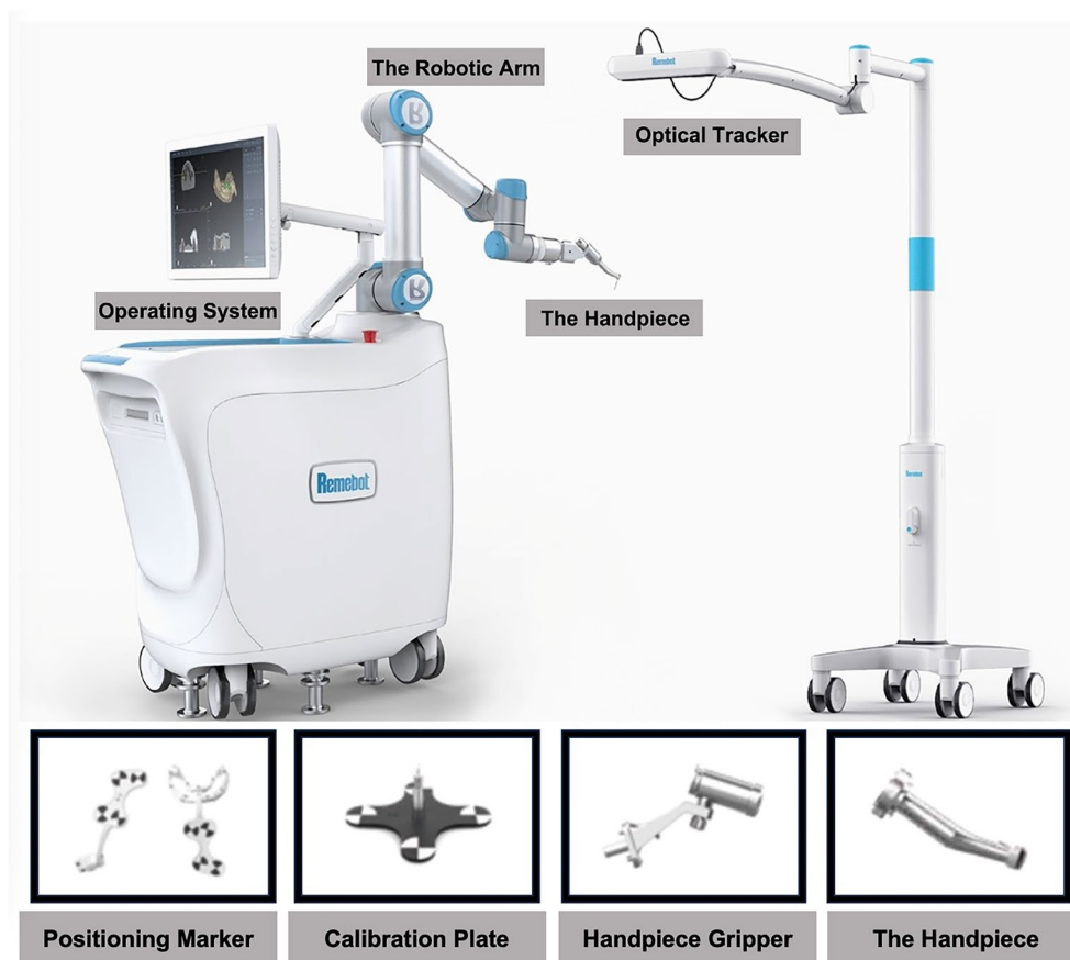
FIGURE 3 The RNS includes an operating system, a robotic arm, and an optical tracker. The accessories of the system include a positioning marker, a calibration plate, a handpiece gripper and the handpiece. Before the operation, calibration was carried out between the calibration plate, which was connected to the handpiece, and the positioning marker, which was fixated on the patient's dentition. By calibration, the position of the targeted tooth can be located by the handpiece. During the surgery, the optical tracker could capture the positioning marker, which guided the movement of the handpiece.
